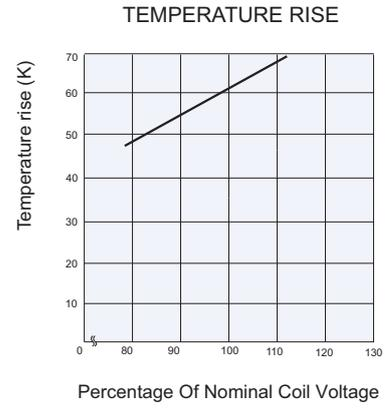
**Test conditions:** Flux proofed, at 85°C
