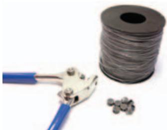
Pliers, steel wire and lead seals used to seal the auxiliary release device (head 96D).
