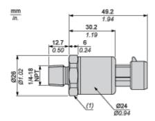
(1) SW24 tightening torque ≤ 25 N.m / 221 lb-in
