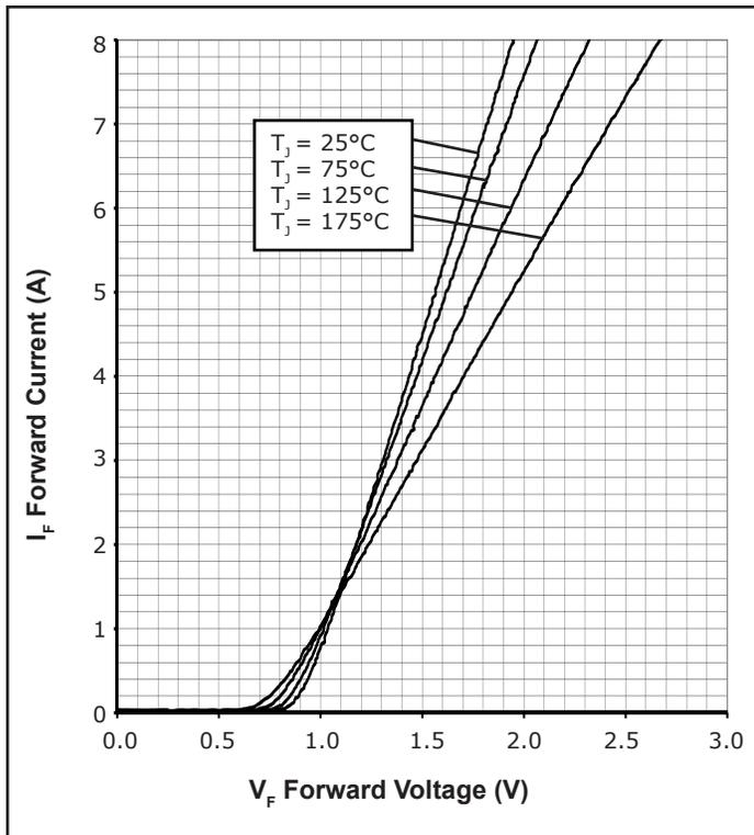
Figure 1. Forward Characteristics
