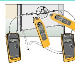
Precise location of cable interruptions with additional transmitter
