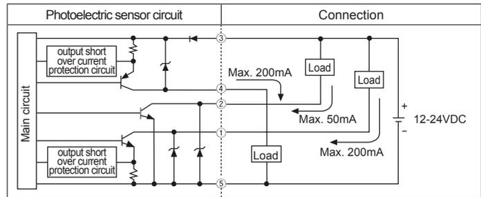
※ In case of product with the output protection device, if terminals of control output are short-circuited or overcurrent condition exists, the control output will turn off due to protection circuit.
