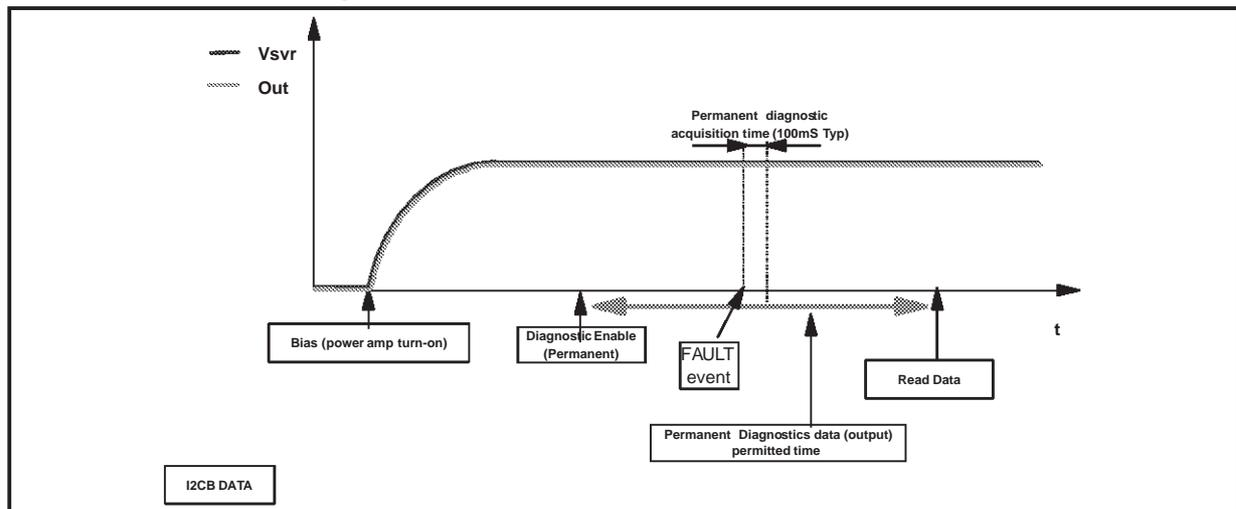
Figure 16. SVR and Output pin behaviour
