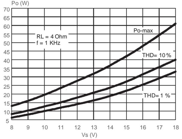
**Figure 4. Output Power vs. Supply Voltage (2Ω)**
