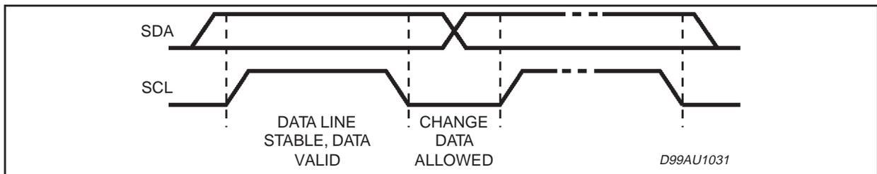
**Figure 20: Timing Diagram on the I<sup>2</sup>C BUS**
