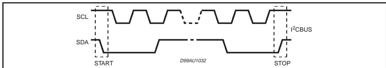
**Figure 21: Acknowledge on the I<sup>2</sup>C BUS**
