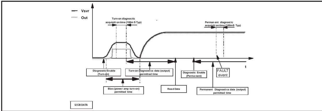
The information related to the outputs status is read and memorized at the end of the current pulse top. The acquisition time is 100 ms (typ.). No audible noise is generated in the process. As for SHORT TO GND / Vs the fault-detection thresholds remain unchanged from 26 dB to 12 dB gain setting. They are as follows:
