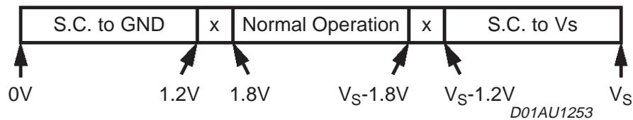
Concerning SHORT ACROSS THE SPEAKER / OPEN SPEAKER, the threshold varies from 26 dB to 12 dB gain setting, since different loads are expected (either normal speaker's impedance or high impedance). The values in case of 26 dB gain are as follows:
