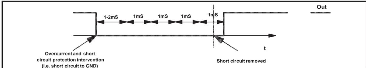
**Figure 18. Restart timing with Diagnostic Enable (Permanent)**
