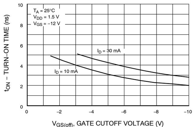
Figure 7. Switching Turn-On Time vs. Gate-Source Cut-Off Voltage
