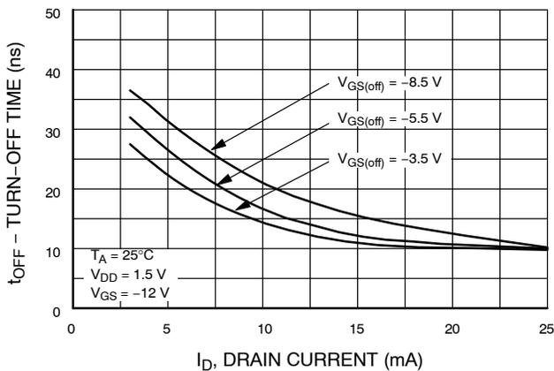
Figure 8. Switching Turn-Off Time vs. Drain Current
