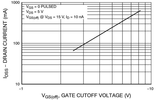
Figure 5. Drain Current vs. Gate-Source Cut-Off Voltage
