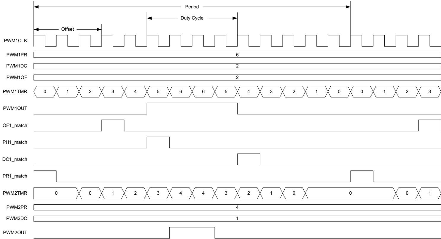
**FIGURE 22-13: OFFSET MATCH ON DECREMENTING TIMER TIMING DIAGRAM**
