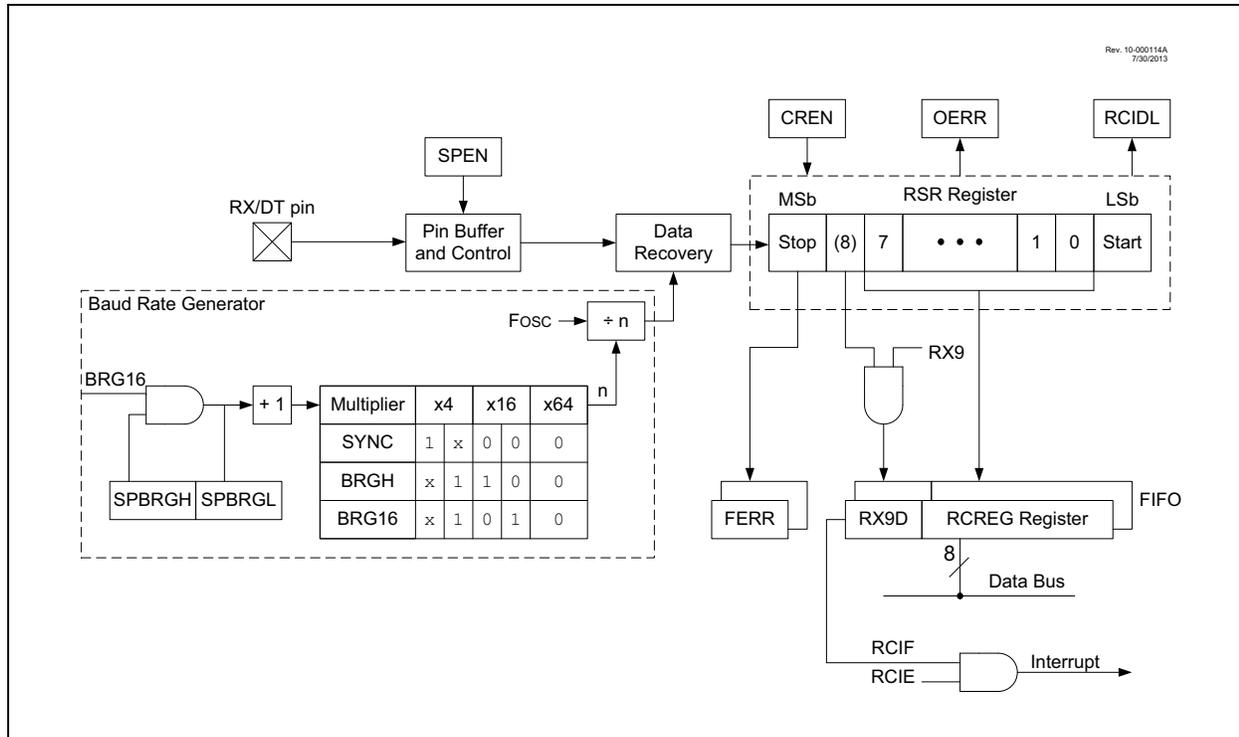
The operation of the EUSART module is controlled through three registers:
