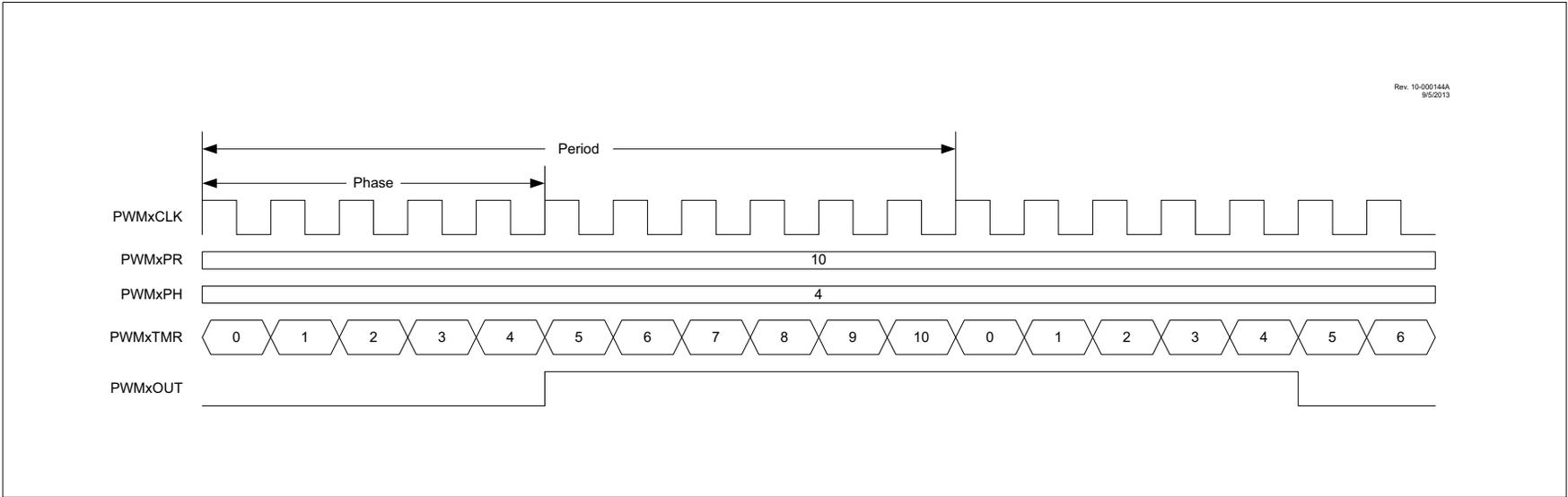
FIGURE 22-7: CENTER ALIGNED PWM MODE TIMING DIAGRAM
