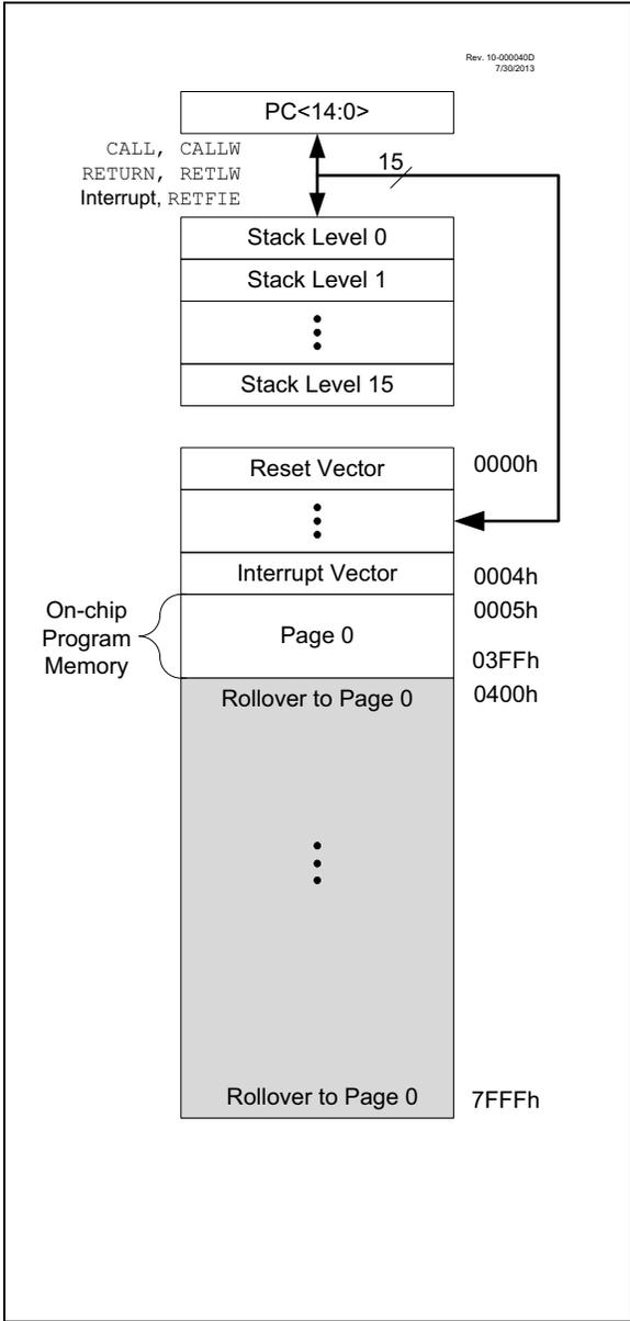
FIGURE 3-2: PROGRAM MEMORY MAP AND STACK FOR PIC12(L)F1572
