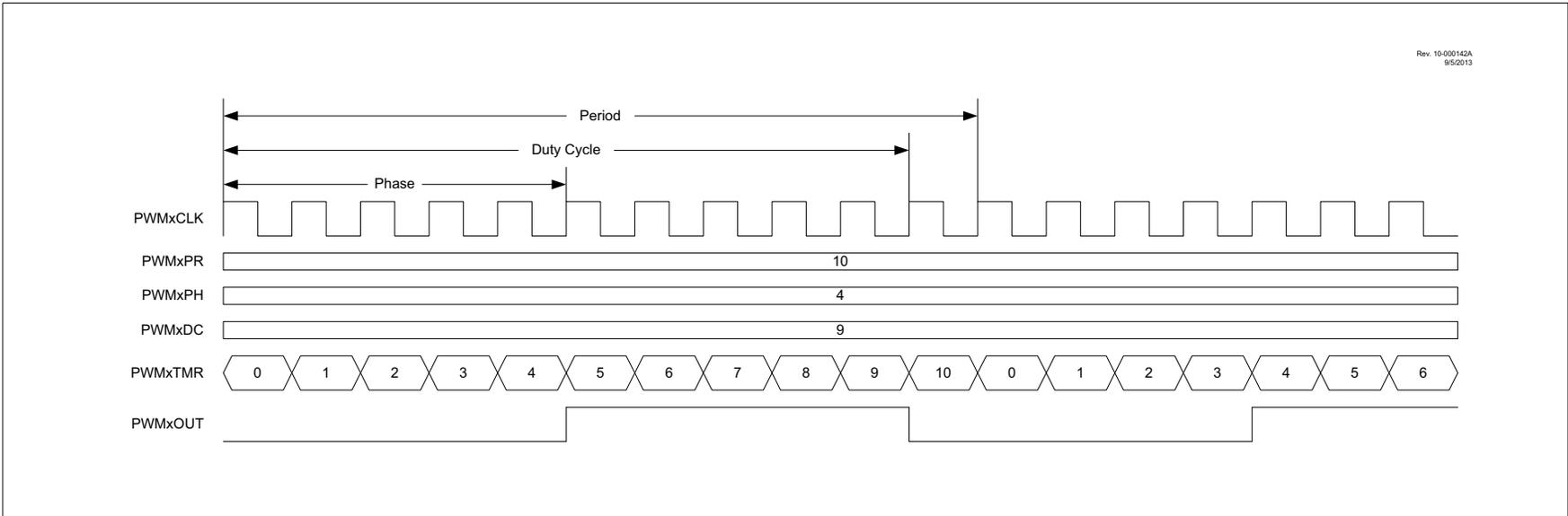
**FIGURE 22-5: SET ON MATCH PWM MODE TIMING DIAGRAM**
