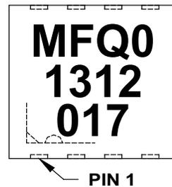
**TABLE 29-1: 8-LEAD 3X3 DFN (MF) TOP MARKING**
