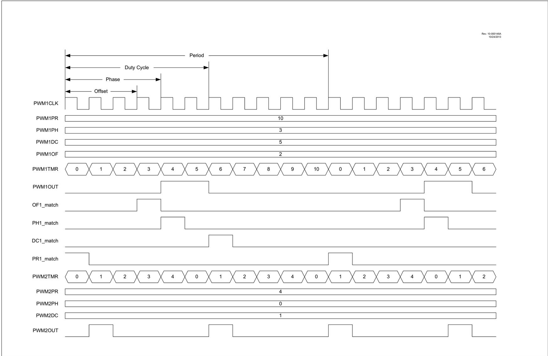
**FIGURE 22-9: INDEPENDENT SLAVE RUN MODE WITH SYNC START TIMING DIAGRAM**
