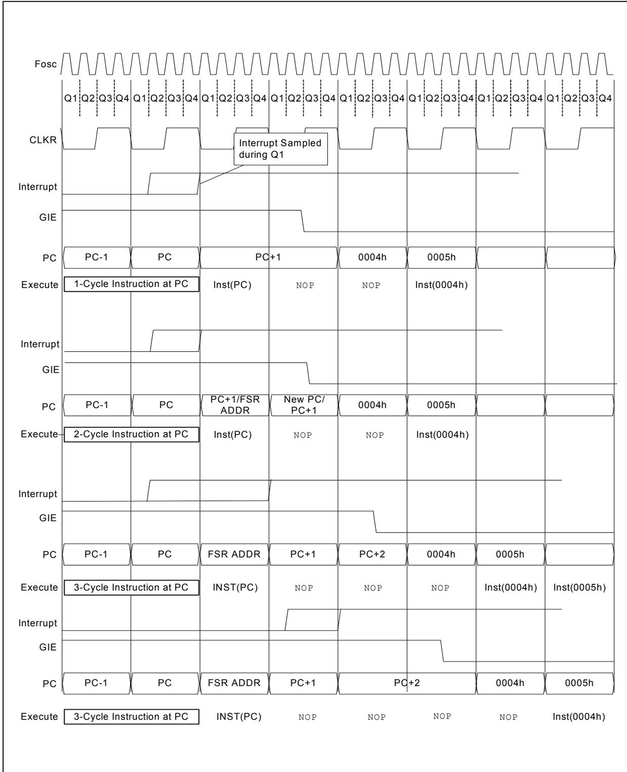
**FIGURE 7-3: INT PIN INTERRUPT TIMING**
