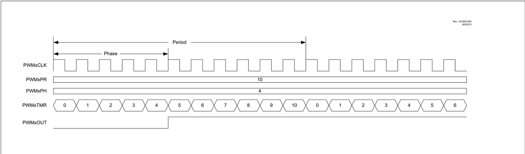
FIGURE 22-6: TOGGLE-ON MATCH PWM MODE TIMING DIAGRAM
