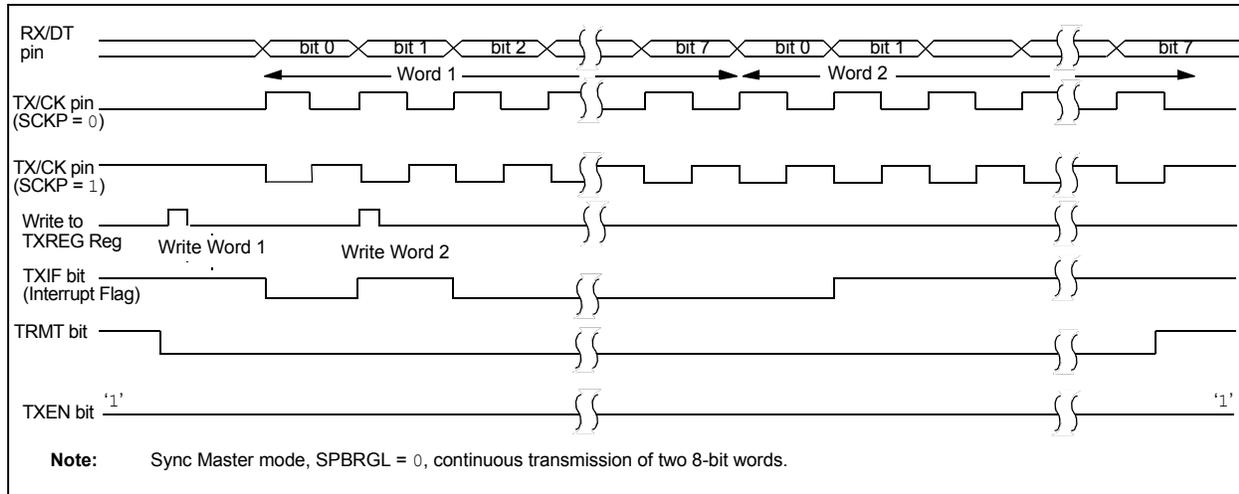
**FIGURE 21-11: SYNCHRONOUS TRANSMISSION (THROUGH TXEN)**
