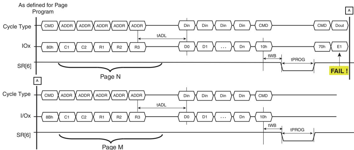
The device supports Random Data Input within a page. The column address of next data, which will be entered, may be changed to the address which follows the Random Data Input command (85h). Random Data Input may be operated multiple times regardless of how many times it is done in a page.
