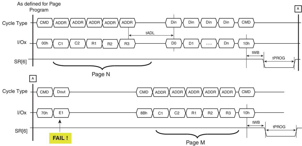
On the other hand, if the pattern bound for the target page is different from that of the previous page, data in cycles can be issued before program confirm '10h', as described in [Figure 3.2](#).
