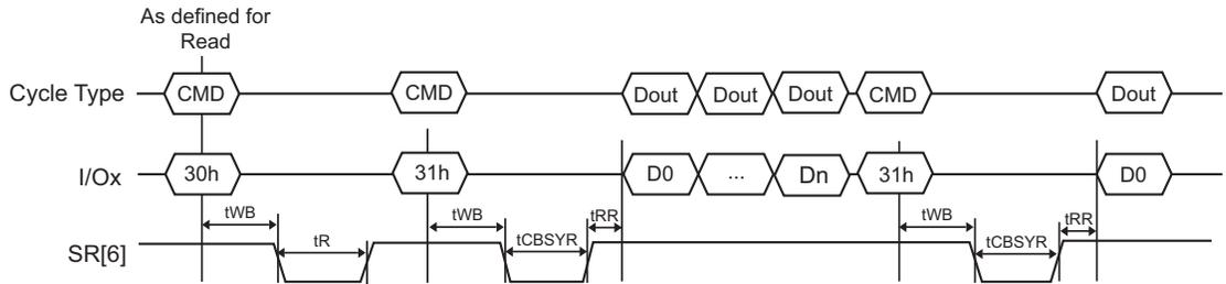
**Figure 6.27** “Random” Read Cache Timing, Start (and Continuation) of Cache Operation
