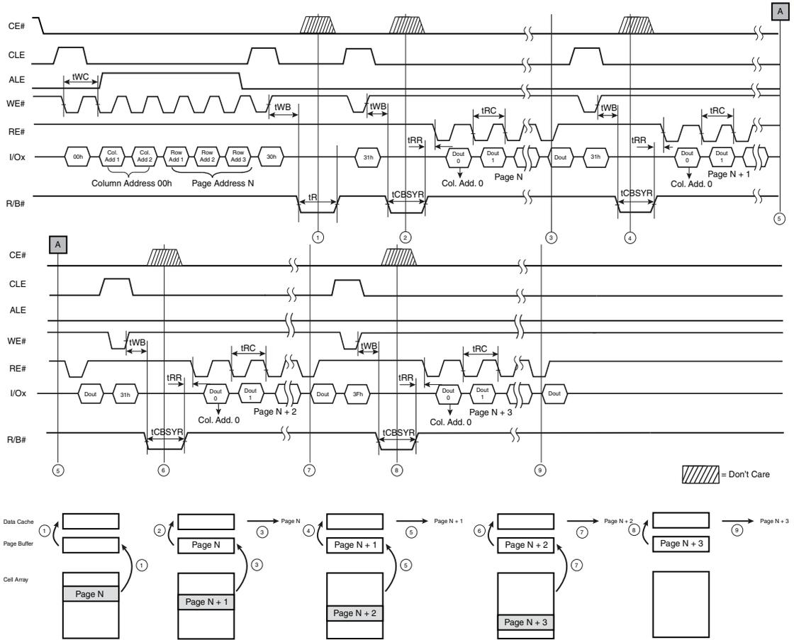
Figure 6.26 “Sequential” Read Cache Timing, Start (and Continuation) of Cache Operation
