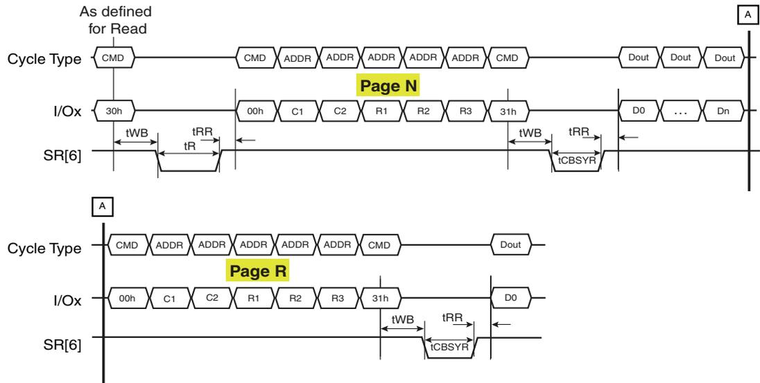
**Figure 6.28** Read Cache Timing, End Of Cache Operation
