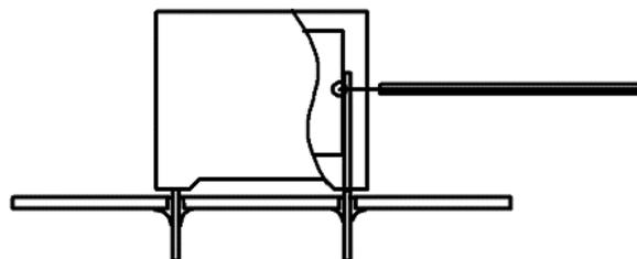
Temperature monitored inside the capacitor.
