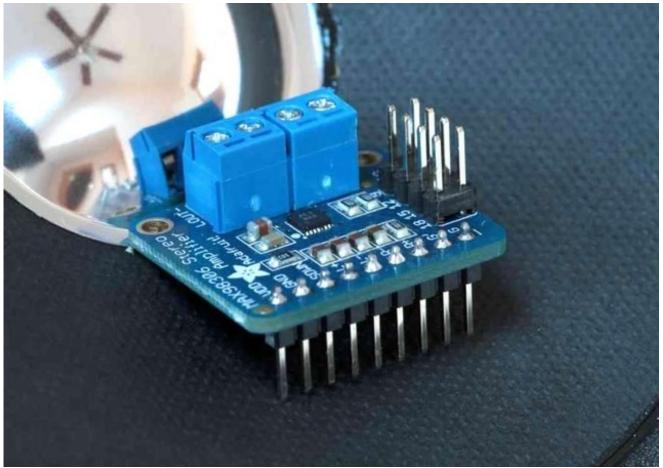
This incredibly small stereo amplifier is surprisingly powerful - able to deliver  $2 \times 3.7W$  channels into 3 ohm impedance speakers. Inside the miniature chip is a class D controller, able to run from 2.7V-5.5VDC. Since the amp is a class D, its incredibly efficient (over 90% efficient when driving an  $8\Omega$  speaker at over a Watt).
