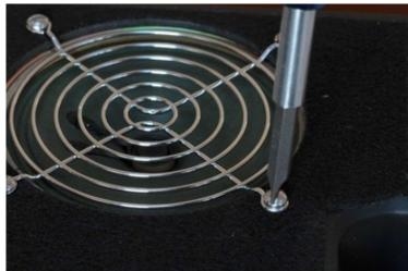
Cut holes in the box to fit your speakers and mount them in the box with screws. Here we used 4" speakers with 4" fan grilles and mounted them with 3/4" 6-32 machine screws and nuts.
