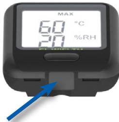
USB port sealed with rubber gasket
