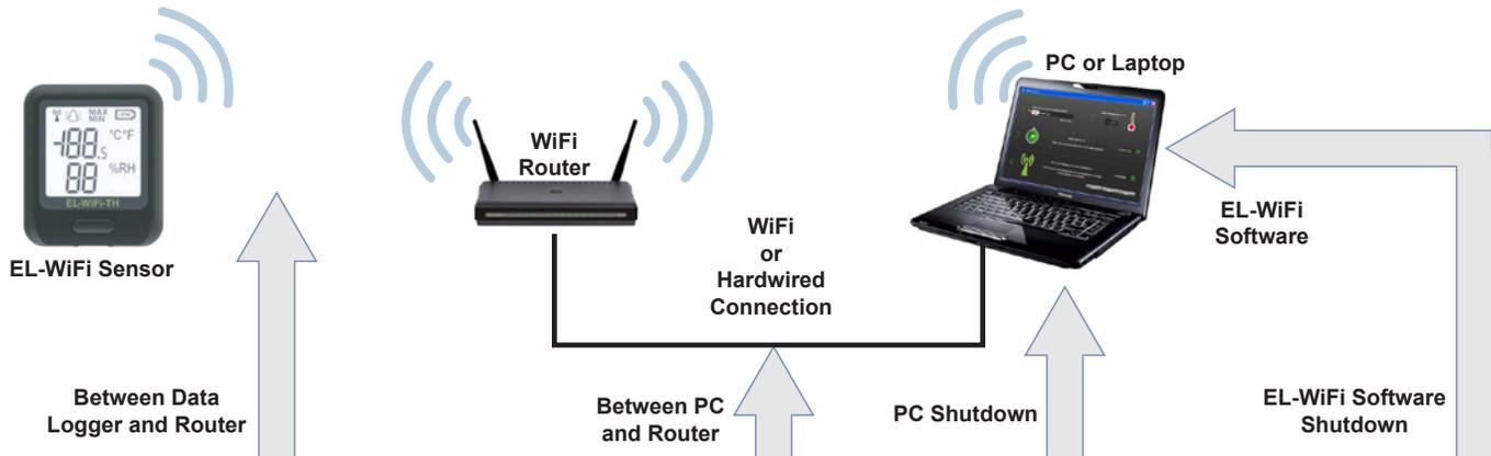
EL-WiFi products support a failsafe operation feature that ensures retained readings and data logging continuity in the event of failure at one or more communication junctions: between the data logger and the WiFi router; between the WiFi router and PC; PC shut down; EL-WiFi software shutdown.
