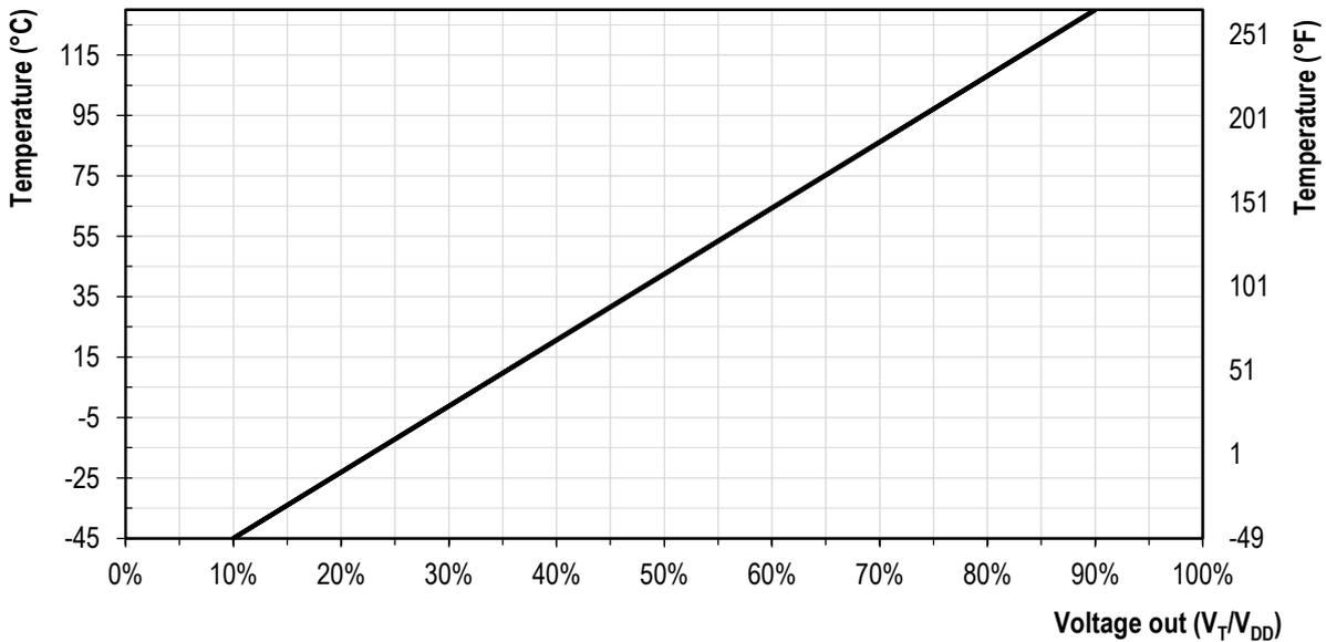
**Figure 9** Relationship between the ratiometric analog voltage output and the measured temperature
