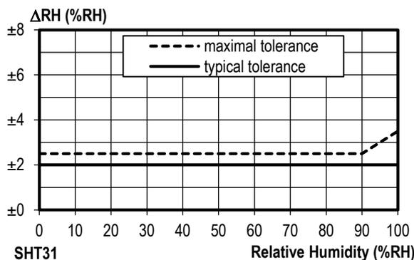
**Figure 4** Tolerance of RH at 25°C for SHT31
