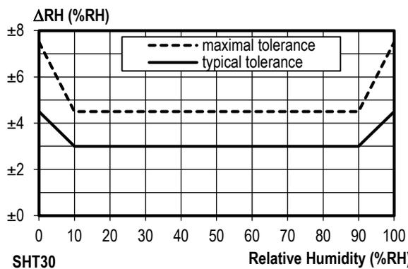
**Figure 2** Tolerance of RH at 25°C for SHT30
