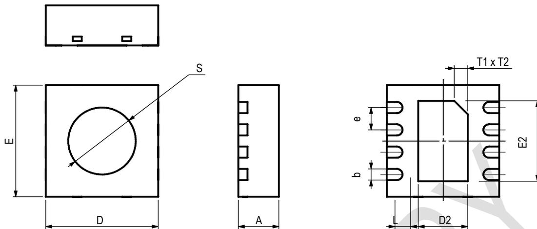
Figure 11 Dimensional drawing of SHT3x-ARP sensor package
