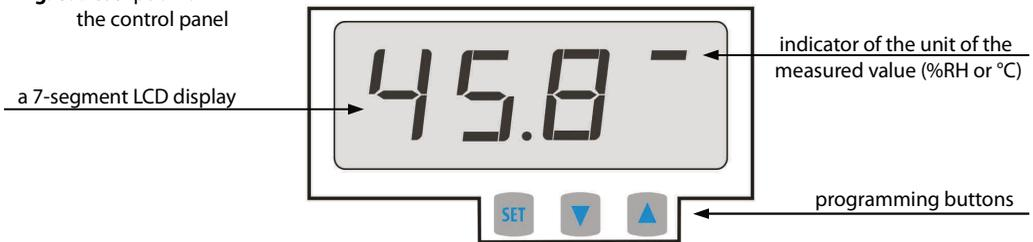
a) button functions in the measurement display mode
