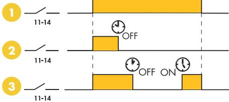
\*Note 3: Depending on the time of year (summer specifically) it may be that the override ON time will fall after the AstroOFF time. In this case, the output switches off at the Astro OFF time and the override ON time is ignored.
