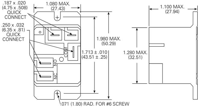
Note: Recommended mounting screw torque is 4.0-5.0 lbs.in when #6 screw is used.
