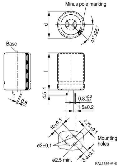
Snap-in terminals, length (6.3 ±1) mm. Also available in a shorter version with a length of (4.5 –1) mm. PET insulation is marked with label "PET" on the sleeve. Safety vent on the base.
