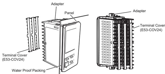
1. For waterproof mounting, waterproof packing must be installed on the Controller. Waterproofing is not possible when group mounting several Controllers. Waterproof packing is not necessary when there is no need for the waterproofing function.
