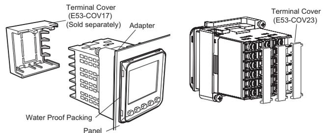
1. For waterproof mounting, waterproof packing must be installed on the Controller. Waterproofing is not possible when group mounting several Controllers. Waterproof packing is not necessary when there is no need for the waterproofing function.
