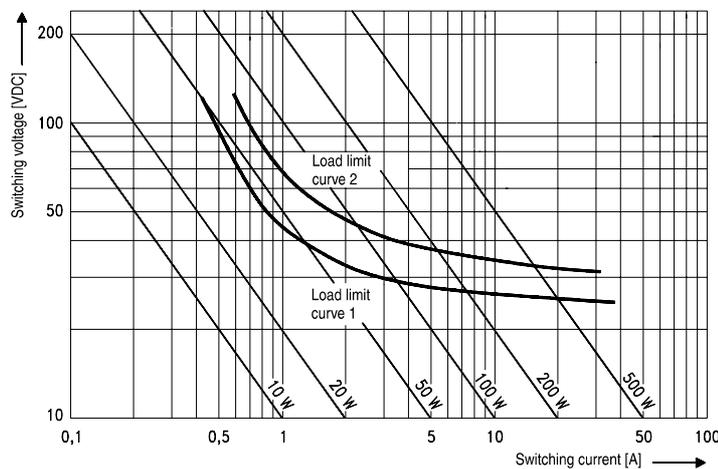
Load limit curve 1 ≙ arc extinguishes, during transit time (changeover contact)
