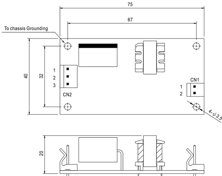
AC Input Connector (CN2) : Molex 5285-03 or equivalent
