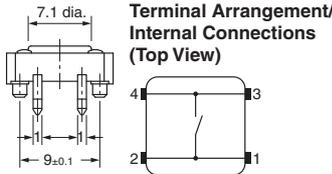
Standard, Long-durability, and High-reliability Models Flat Plunger Type (with Ground Terminal)
