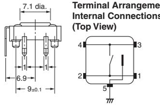
Standard, Long-durability, and High-reliability Models Projected Plunger Type (without Ground Terminal)
