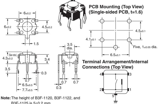
**Note:** The height of B3F-1120, B3F-1122, and B3F-1125 is  $5 \pm 0.2$  mm.
