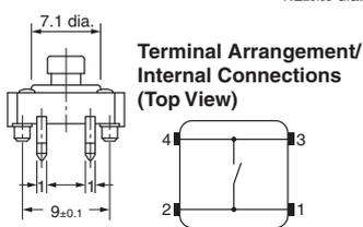
Standard, Long-durability, and High-reliability Models Projected Plunger Type (with Ground Terminal)
