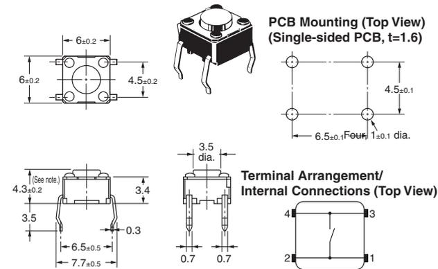
**Note:** The height of B3F-1020, B3F-1022, B3F-1025, and B3F-1026 is  $5 \pm 0.2$  mm.
