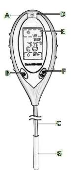
A. PH/ TEMP KEY: mode switch: Set the mode for PH value, temperature or moisture.
