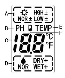
A. Sunlight intensity display area: 9 levels: LOW-, LOW, LOW+, NOR-, NOR, NOR+, HGH- ,HGH, HGH+,each increasing in amount and quality. LOW- signifies an extremely dim environment. HGH+ signifies an extremely bright environment.
