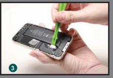
The prying paddle and opening levers are made of Polyoxymethylene (POM) to prevent scratching or chipping your plastic case, Ideal for used by Apple professionals to safely open laptops, iPods, iPads, & iPhones or other electronic devices.
