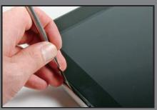
The double-ended metal spudger is widely use to open cases that require more leverage or a sharper tip. Handy for cell phones, laptops, LCD screens, and other plastic electronics.
