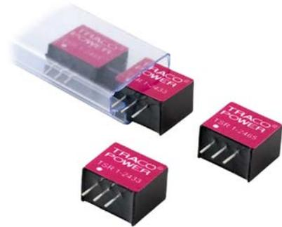
The new TSR-1 series step-down switching regulators are drop-in replacement for inefficient 78xx linear regulators. A high efficiency up to 96 % allows full load operation up to  $+60^{\circ}\text{C}$  ambient temperature without the need of any heat-sink or forced cooling.
