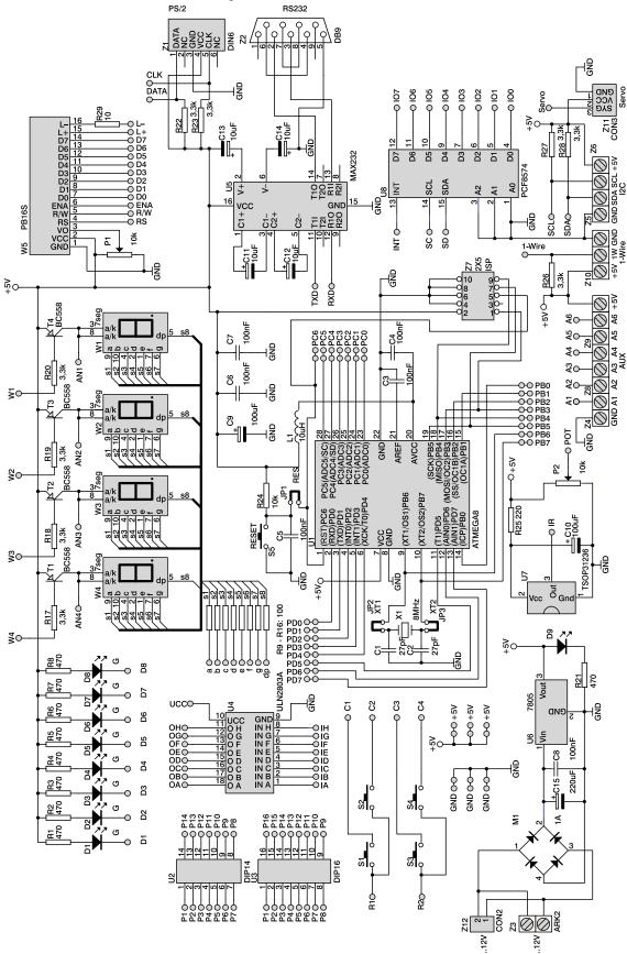
Fig. 1. Circuit diagram of ZL2AVR
