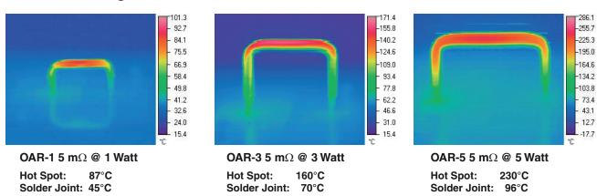
The thermal images (not simulations) above are of the OAR products at their respective power rating. Notice the solder joint temperature is much lower than the hotspot. The unique construction of the OAR isolates the temperature of the hotspot from the circuit board material preventing damage to the circuit board. Additionally, the thermal energy is dissipated to the air instead of being conducted into the circuit board potentially causing a nearby power component to exceed its rating.
