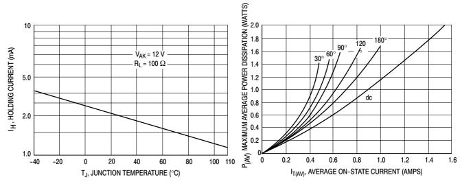
Figure 7. Typical Holding Current
