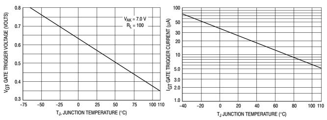
Figure 5. Typical Gate Trigger Voltage
