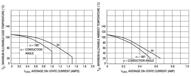
Figure 1. Maximum Case Temperature
