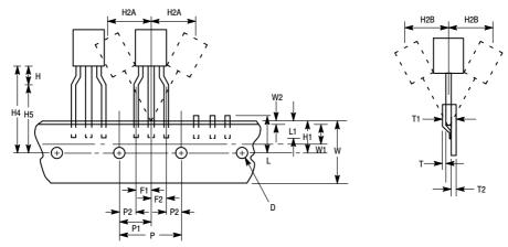
Figure 9. Device Positioning on Tape
