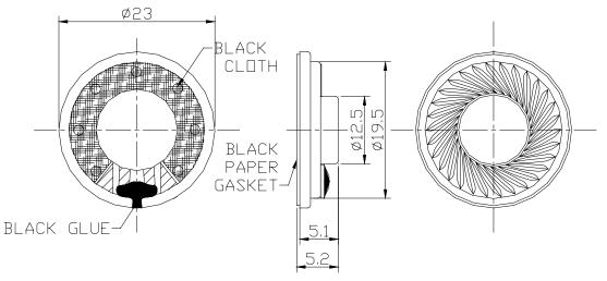
Dimensions : Millimetres Tolerance: ±0.5mm
