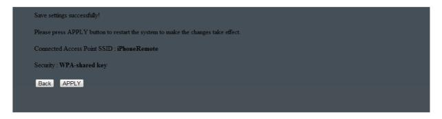
If the key was Correct the client has saved the settings and displays the network name of the access point it will connect to. Click 'Apply' to restart the device with the new settings.
