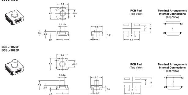
$\textbf{Note:} \quad \text{Unless otherwise specified, a tolerance of $\pm 0.4$ mm applies to all dimensions. No terminal numbers are indicated on the Switches.}$
