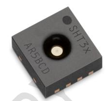
processing, temperature and humidity can be read out at different pins. The DFN package has a footprint of 2.5 x 2.5 mm while keeping a height of 0.9 mm. This allows for integration of the SHT3x-ARP into a great variety of applications. Additionally, the wide supply voltage range of 2.4 to 5.5 V guarantees compatibility with diverse assembly situations. All in all, the SHT3x-ARP incorporates 15 years of knowledge of Sensirion, the leader in the humidity sensor industry.
