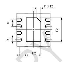
Figure 11 Dimensional drawing of SHT3x-ARP sensor package
