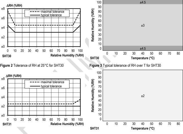
Figure 4 Tolerance of RH at 25°C for SHT31
