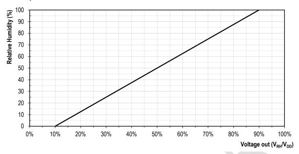
Figure 8 Relationship between the ratiometric analog voltage output and the measured relative humidity
