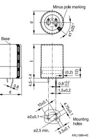
Snap-in terminals, length (6.3 + 1/-1.4) mm. Also available in a shorter version with a length of (4.5 - 1.4) mm. PET insulation cap is positioned under the insulation sleeve. Safety vent on the base.
