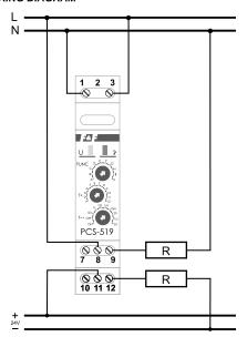
An example of the power supply system by 230V of relay which control the receiver powered by 230V and 24 V
