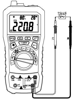
Do not allow measurement of any voltage higher than DC 1000V or AC 750VRMS, otherwise it may cause instrument damage, electric shock or personal injuries.
