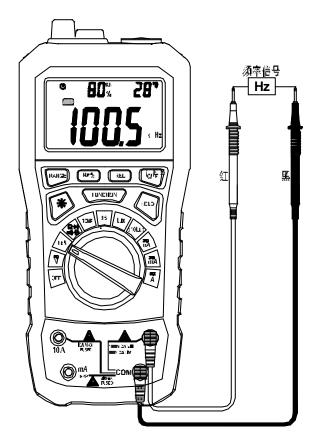
3. Contact the probe to the measured circuit, and measure the frequency.
