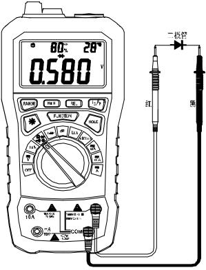
2. Insert the red probe in "" socket, and the black probe in "COM" socket.
