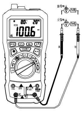
rotary knob to any shift among "A", "A" and "A", press "FUNCTION" button and switch to AC or DC function.
