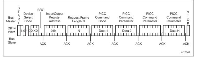
Figure 14. CR14-to-Host Transfer: I<sup>2</sup>C Random Address Read from Input/Output Frame Register for ISO14443B
