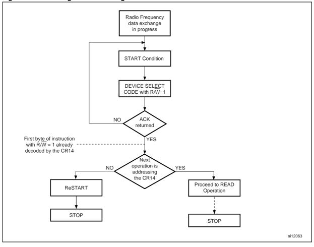
Figure 8. I<sup>2</sup>C Polling Flowchart using ACK
