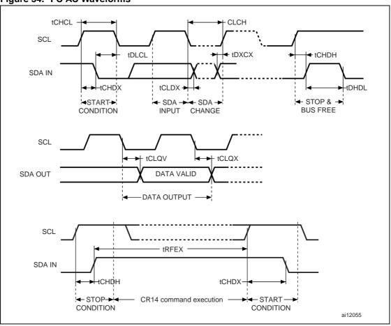
Figure 34. I<sup>2</sup>C AC Waveforms
