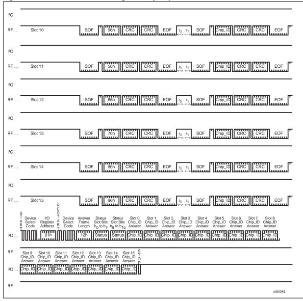
Figure 32. Anti-Collision ST short range memory Sequence Continued
