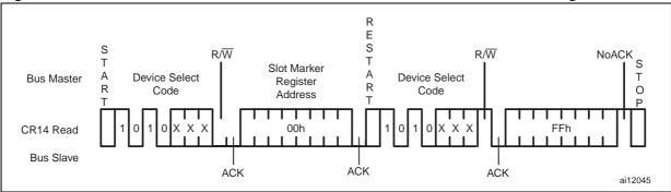
Figure 17. CR14-to-Host Transfer: I<sup>2</sup>C Random Address Read from Slot Marker Register
