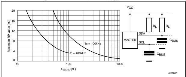
Figure 5. Maximum  $R_L$  Value versus Bus Capacitance ( $C_{BUS}$ ) for an I<sup>2</sup>C Bus
