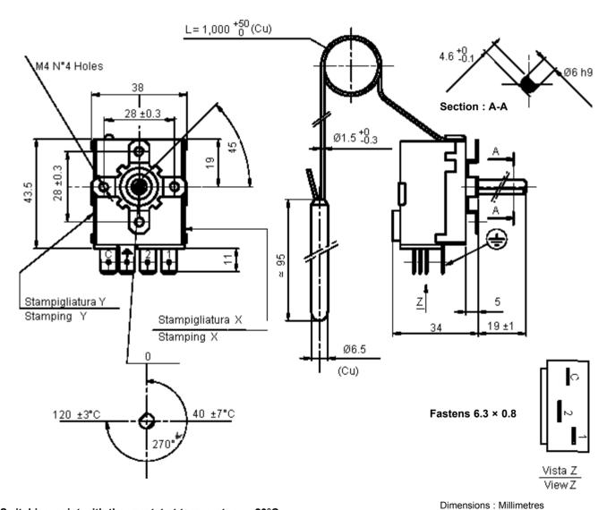
Switching point with thermostat at temperature = 20°C.
